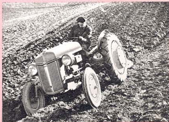
On hillsides, there is no doubt about the extra stability provided by the Ferguson system and 4-wheel Ford tractor.
