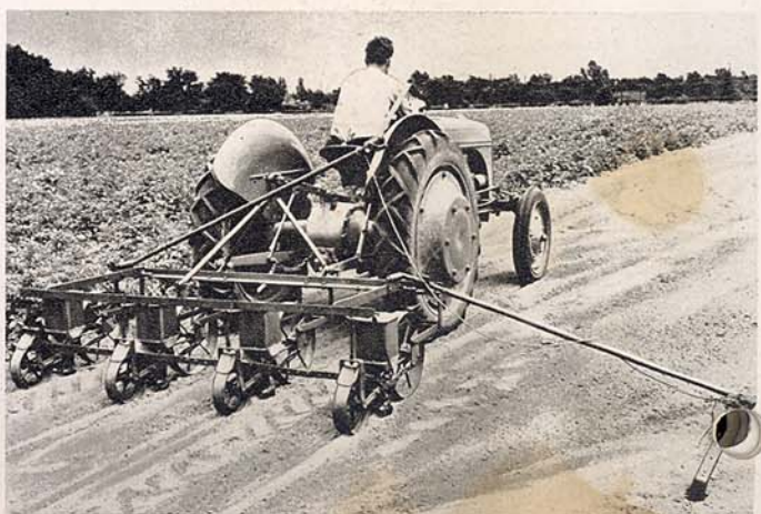
Four-row vegetable and beet planter for the Ford tractor.
