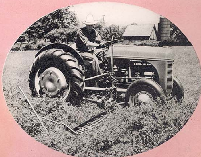
A touch on the finger-tip hydraulic control lever lifts cutterbar on the Detroit Highway and heavy-duty farm mower for the new Ford tractor to any position from vertical to 45° below horizontal. Sickle operates in any of these positions.
