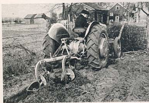
Younger members of the family easily operate the new Ford tractor with Ferguson system finger-tip hydraulic control.
