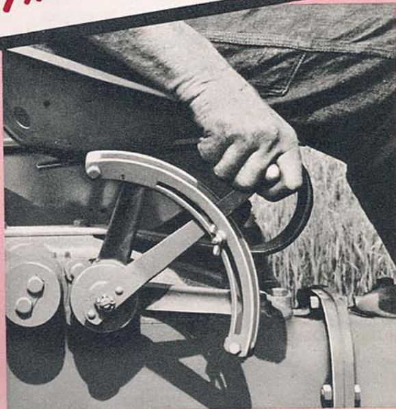
Raising, lowering and setting the depth of the implement are the simplest operations you can imagine with this hydraulic control lever. A stop on the quadrant is adjustable for various depths.
